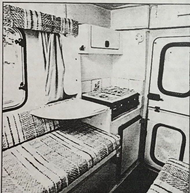
Fold-down shelf (left) provides work surface. Roof lockers (below left) are top hinged. Inboard water tank and storage space (below) in seat base
