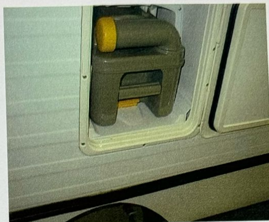
16 View showing Casset for Toilet
