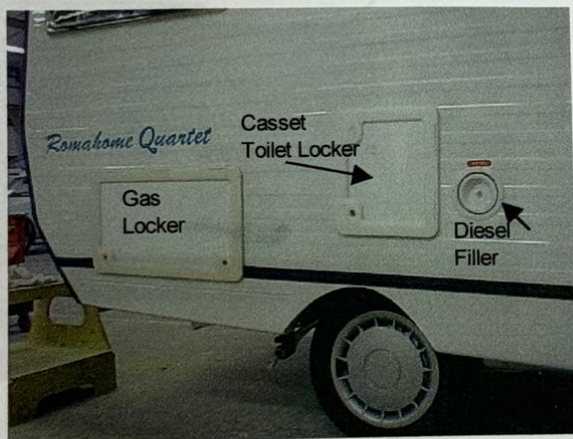
11 View showing near-side lockers
